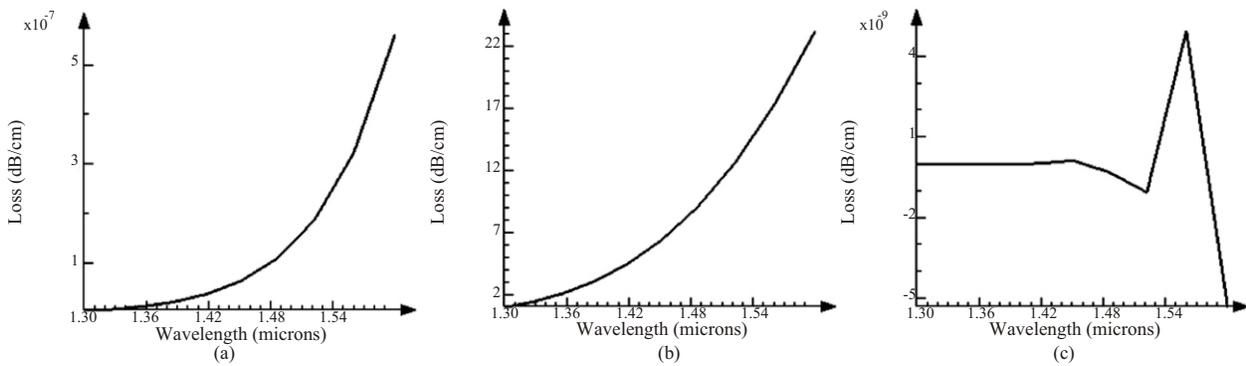
Fig. 3. Comparison of confinement losses for the three designs of HC-PCF
